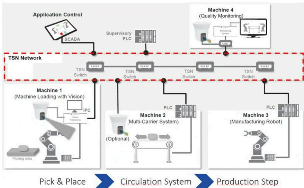
Figure 1 Production Lines Use case
